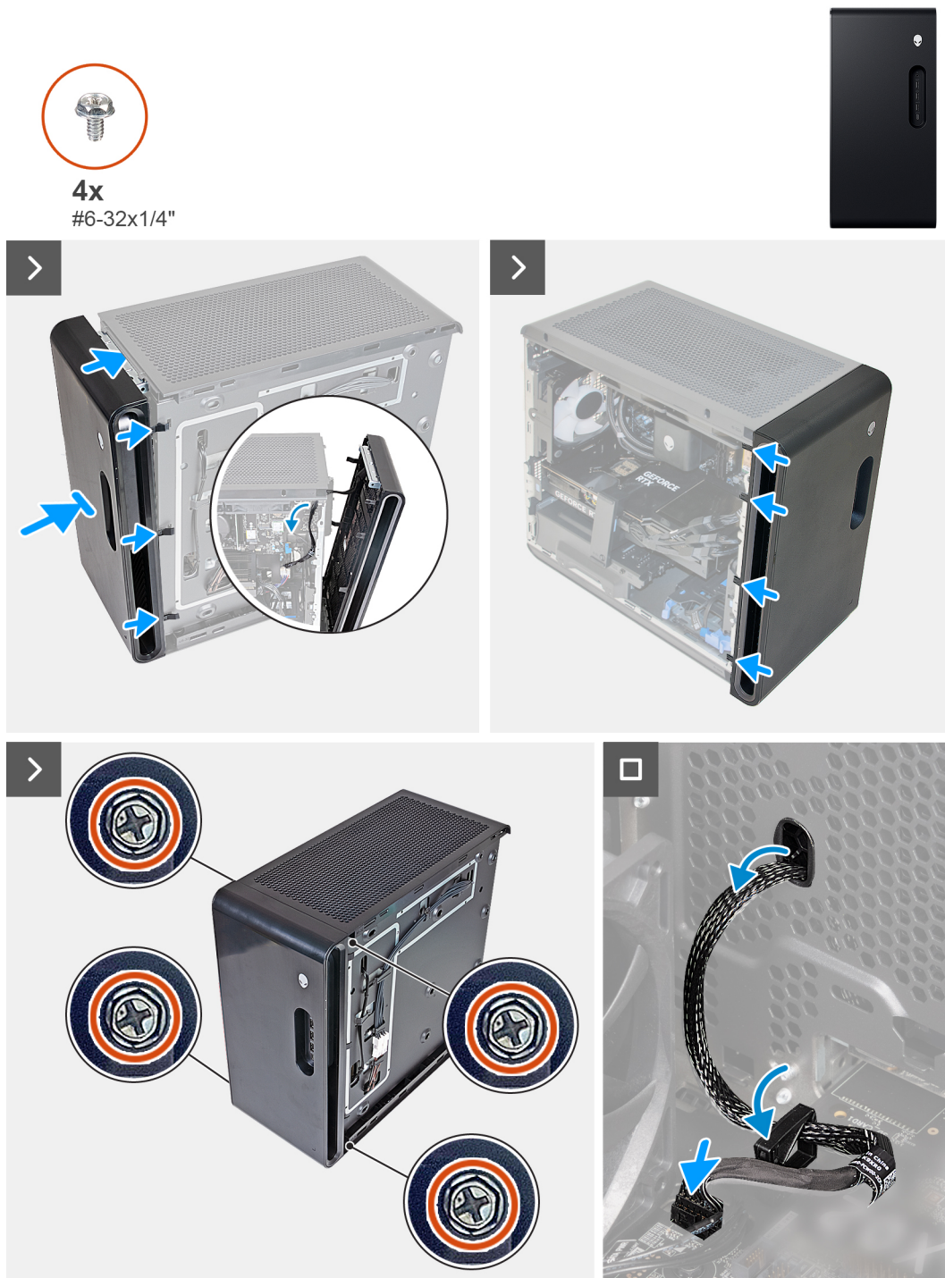
Figure 19. Installing the front bezel
