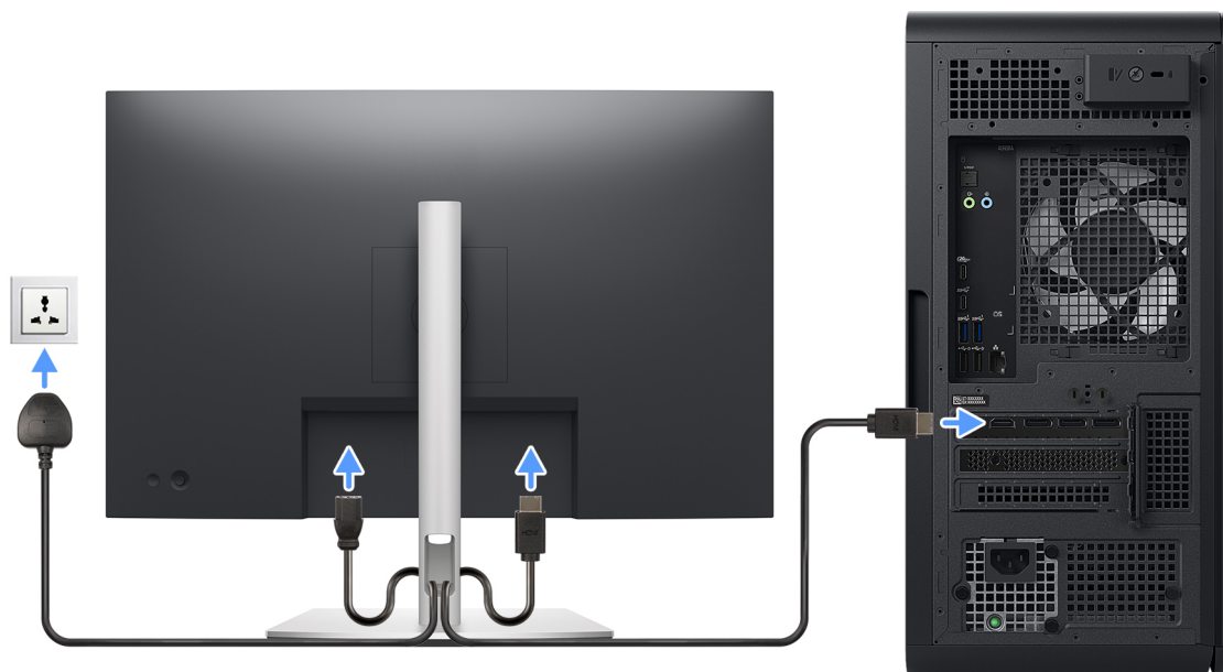
Figure 9. Connecting the display
