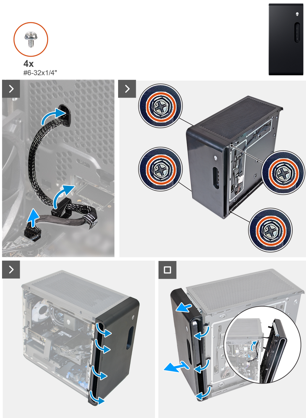
Figure 18. Removing the front bezel
