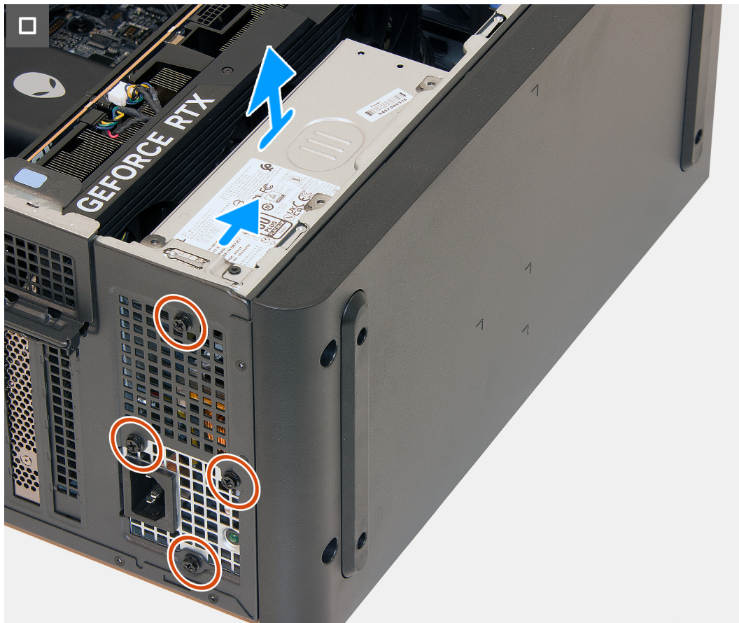
Figure 46. Removing the power-supply unit
