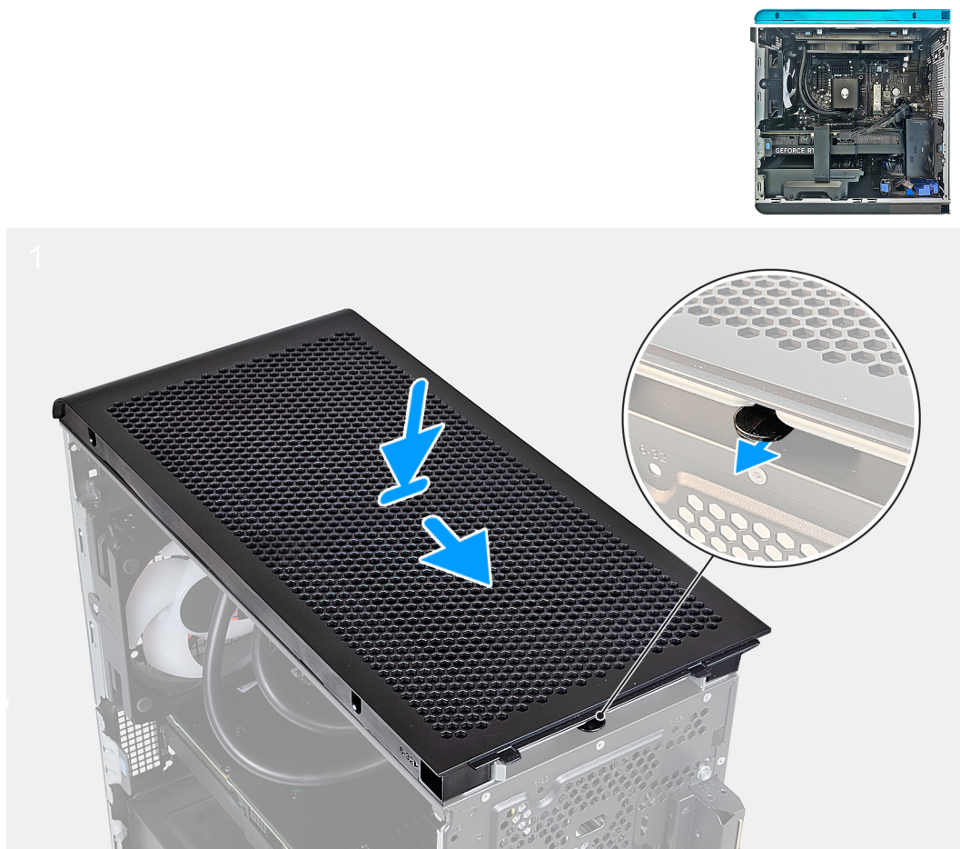
Figure 21. Installing the top cover
