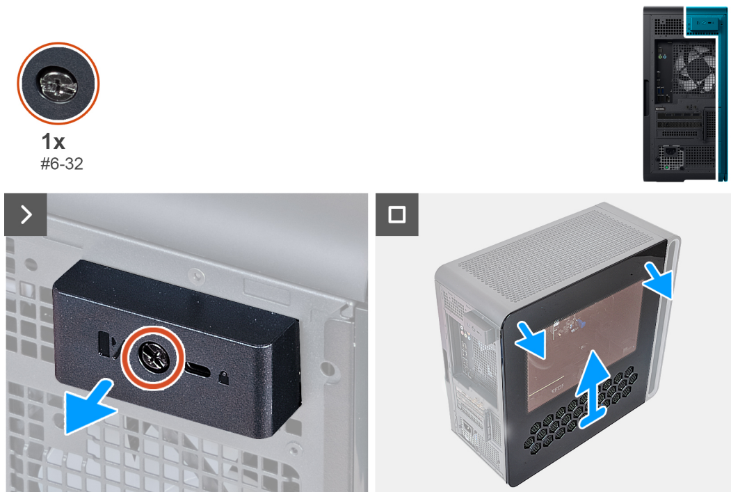
Figure 14. Removing the left-side cover
