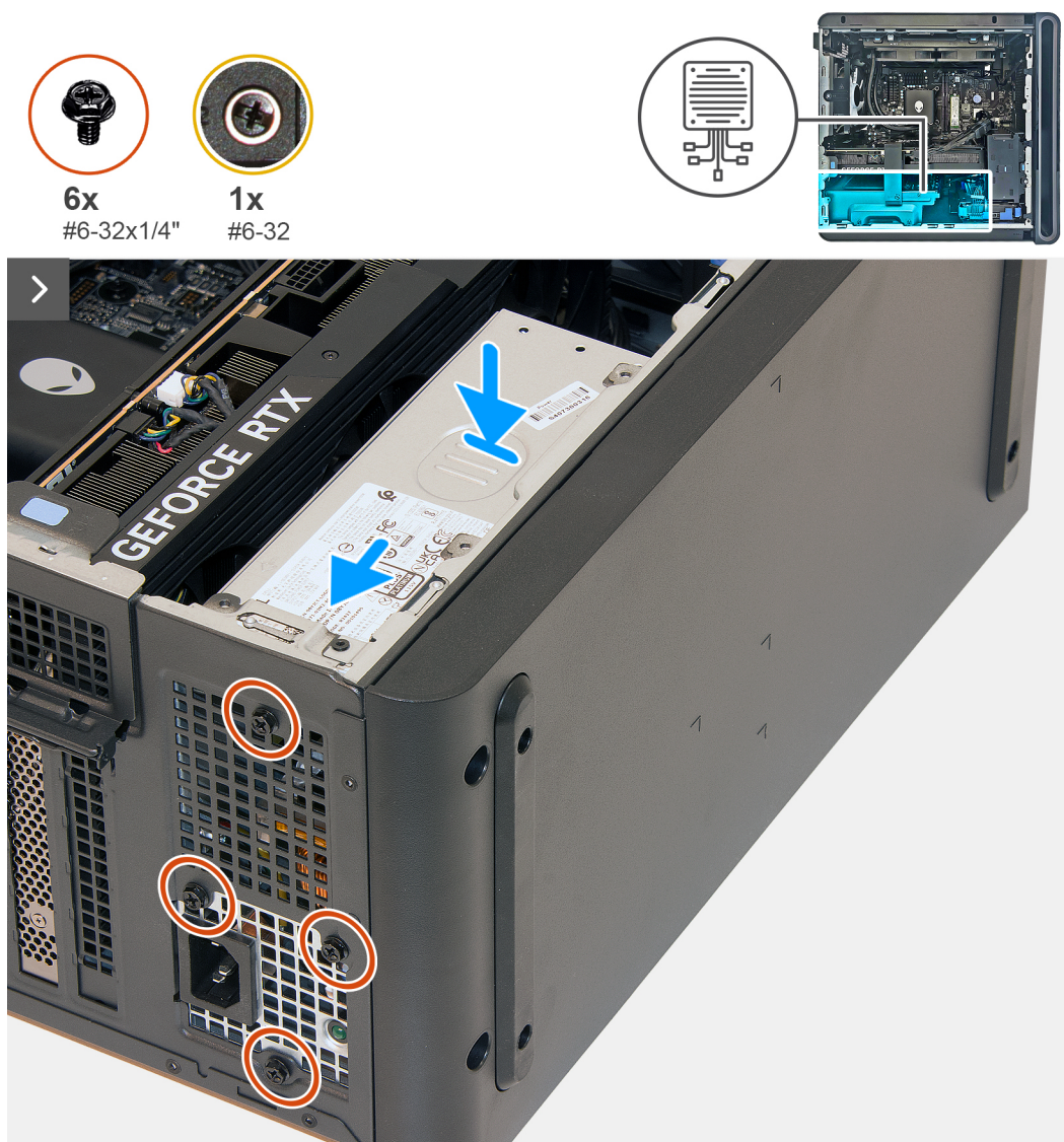
Figure 47. Installing the power-supply unit
