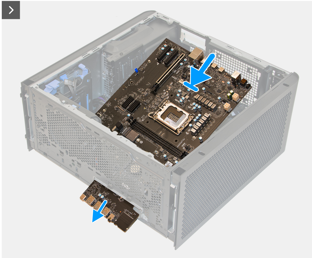
Figure 67. Installing the system board
