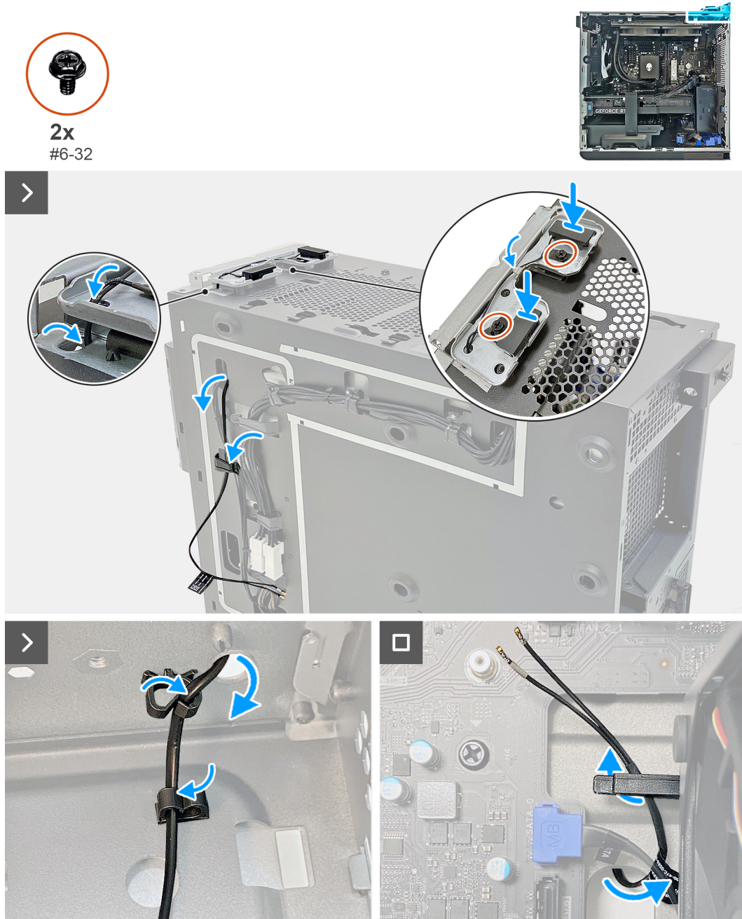
Figure 58. Installing the antenna
