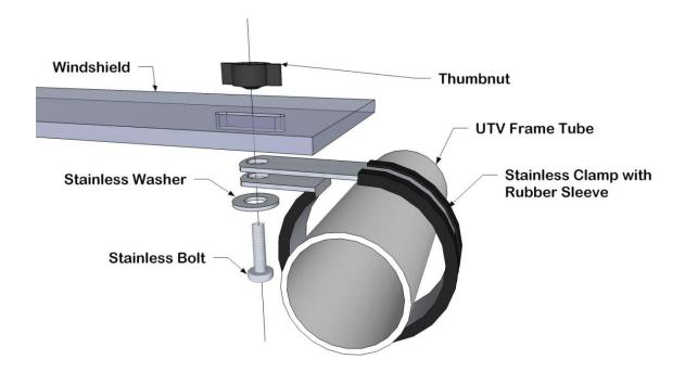
5. Now move to the top section of the windshield and install the bent brace to the top of the windshield if needed. This brace is intended to be used to seal off the front of the cab enclosure that is manufactured by Falcon Ridge. If it interferes with any accessories that are installed on your vehicle please leave off. It should be installed as shown below.
