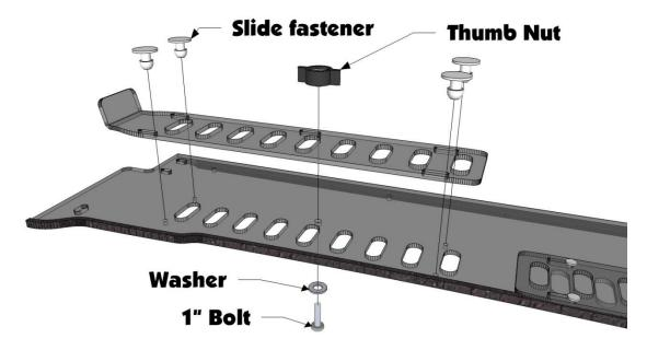
4. Now clamp the bottom section to the Teryx. The windshield should be clamped as shown in the image below.
