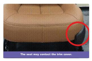
A squeak, scrape, or rub-type noise may be heard coming from the seat area on some 2013 Verano models with a manual transmission (RPO MYJ). The noise will only be heard during a clutch pedal apply.
