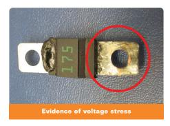
If the fuses are within specifications, inspect around the edge of the black plastic portion of these fuses for any sign of
