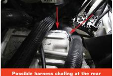
rib of the transmission, viewed from the top of the engine compartment.
