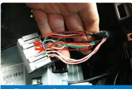
The two tan audio circuits are incorrectly inserted into the radio connector.
