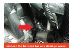
On vehicles with a state-specific emissions system (California, Connecticut, Delaware, Maine, Maryland, Massachusetts, New Jersey, New York, Oregon, Pennsylvania, Rhode Island, Vermont and Washington), the harness at the left rear side of the front cylinder head is not secured by a tie-strap. which may allow the harness to rub on the engine cylinder head.
