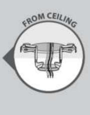
CONNECT WIRES FROM RECEIVER AND FAN TO WIRES FROM OUTLET BOX - Using the wire connectors, connect the brown (live in) wire from the ceiling to the brown wire from the receiver. Connect the blue (neutral) wire from the ceiling to both the blue wire from the receiver and the blue wire from the fan.
