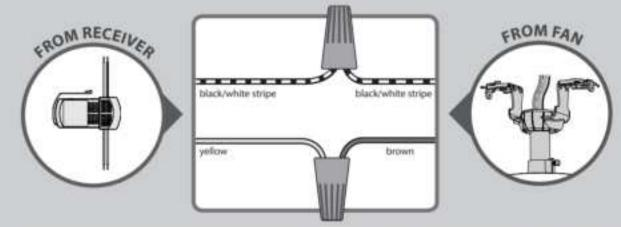
CONNECT WIRES FROM RECEIVER TO FAN - Using the wire connectors, connect the black and white wire from the receiver to the black and white wire from the fan. Connect the yellow wire from the receiver to the brown wire from the fan.
