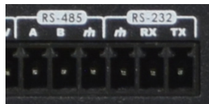
Fig. 11 RS-232 &amp; RS-485 control Ports
