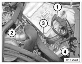
Unlock connector (1) and remove.
