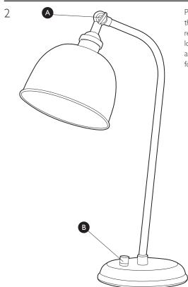
Plug the table lamp into the mains. Switch on using the rotary dimmer switch (B). Your table lamp is now ready for use. The angle of the light can be adjusted by loosening the adjustment key (A), changing the angle, and then re-tightening the key. Allow the shade to cool for 10 minutes prior to adjusting the shade.
