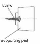
3. Make screw in alignment with the hole on lower base cover. Fasten supporting pad to the base cover firmly by a cross screwdriver (self-provided).
