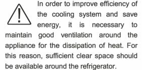
**Suggestion:** It is advisable for there to be at least 50-70mm  $(1.97 \sim 2.76')$  of clearance from the back of the fridge to the wall, at least 100mm (3.94') of clearance from its top, at least 100mm (3.94') from its side to the wall and a clear space in front to allow the doors to open  $135^\circ$ . As shown in following diagrams.
