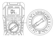
2. Insert the red test lead into the " $V^{\frac{1}{2}+0}_{\Omega MA}$ " terminal and the black test lead into the "COM" terminal.
