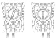
3. Press the "FUNC" Button to measure DC/AC current.
