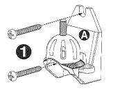
2. Determine the desired orientation (horizontal or vertical) for the speaker. Attach the Mounting Cup Bracket (B) to the indentation (C) on the back of the speaker enclosure using the two supplied M5 screws as shown.
