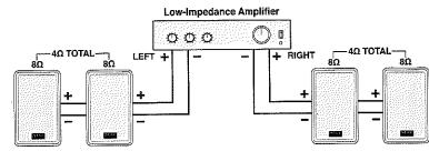
**EXAMPLE:** Two  $8\Omega$  speakers in parallel =  $4\Omega$ . The amplifier must be rated to work into  $4\Omega$  loads. Also in this example, the max amplifier output power rating (each channel into  $4\Omega$ ) should not exceed 150W for S4/T (2 X 75W) speakers or 300 for S5/T (2 X 150W).
