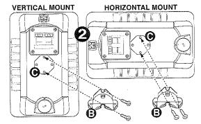
3. Connect the speaker wires to the rear input terminals on the loudspeaker. Set the speaker with Mounting Cup Bracket (B) over the Mounting Base (A). Loosely screw the Mounting Cap Nut (D) onto the Mounting Base threaded stud.
