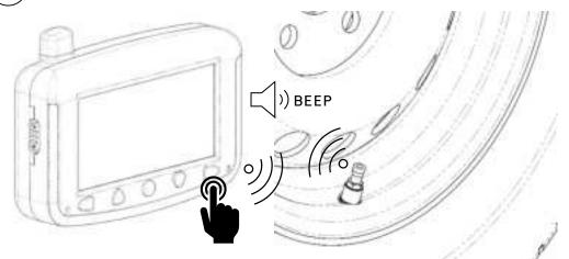
WITH THE MONITOR PREPPED AND THE DISPLAY SHOWING "FFF FFF" POSITION THE MONITOR WITHIN 50cm OR LESS OF THE SENSOR
