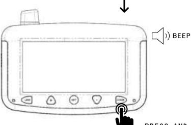
PRESS AND *HOLD* THE "CODE" BUTTON FOR 4-5 SECS
