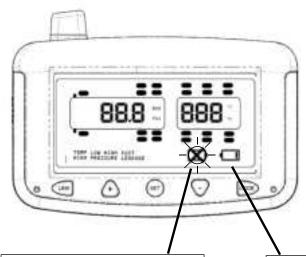
THIS ICON FLASHES WHEN THE SENSOR BATTERY VOLTAGE IS LOW.
