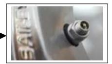
ATTACH THE THREADED COLLAR WITH HEXAGON UPPERMOST, AS SHOWN
