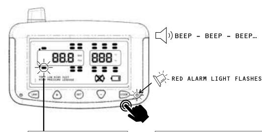
TYRE ICON FLASHES CORRESPONDING TO SENSOR THAT HAS DETECTED AN ALARM
