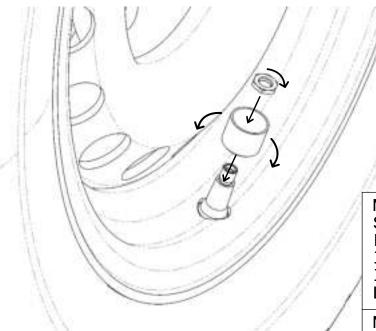
NOTE: WHEN THE DUST SHIELD IS FITTED FOLD IT BACK ON ITSELF. THIS MAKES IT EASIER TO FIT LOCK NUT AND SENSOR.
