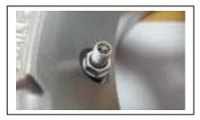
TORQUE THE THREADED COLLAR TO 6.8Nm. REFIT THE TYRE & INFLATE
