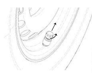
REMOVE SENSOR FROM TYRE VALVE. MONITOR WILL ALARM. REPLACE SENSOR TO CANCEL ALARM. MONITOR WILL THEN SHOW TYRE PRESSURE READING.
