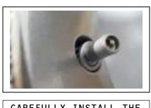
CAREFULLY INSTALL THE WASHER AND ENSURE IT IS SEATED CORRECTLY
