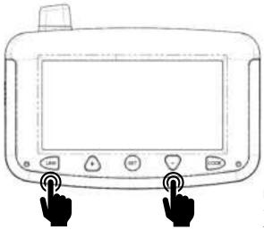
PRESS THE "LINK" AND "-" BUTTON SIMULTANEOUSLY
