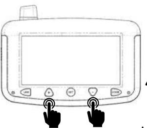
IF YOU WANT TO ADJUST THE FRONT AXLE HIGH PRESSURE ALARM PRESS THE + OR - BUTTONS TO RAISE OR LOWER IT. IF NOT KEEP QUICKLY PRESSING THE SET BUTTON FOR 1 SEC UNTIL THE AXLE YOU WANT IS FLASHING.
