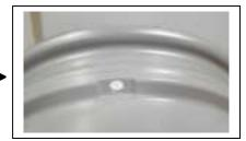
REMOVE OLD VALVE STEM AND CLEAN VALVE STEM HOLE AND MOUNTING FACES
