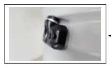
INSTALL SENSOR THROUGH VALVE STEM HOLE FROM INSIDE THE RIM
