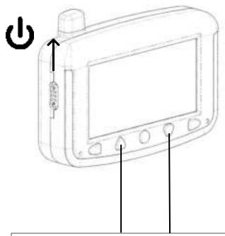
USE "+" OR "-" BUTTON TO SCROLL THROUGH TYRE ICONS TO CHECK PRESSURES AND TEMPERATURES
