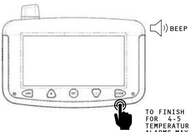
TO FINISH PRESS AND HOLD "CODE" BUTTON FOR 4-5 SECS. TYRE PRESSURES AND TEMPERATURES WILL APPEAR ON THE SCREEN. ALARMS MAY SOUND. THESE CAN BE ADJUSTED DURING THE NEXT STEPS
