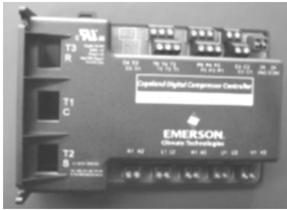
Figure 47 — Variable Capacity Compressor Controller
