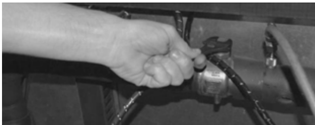
Figure 51 — Remove bolts from suction filter
