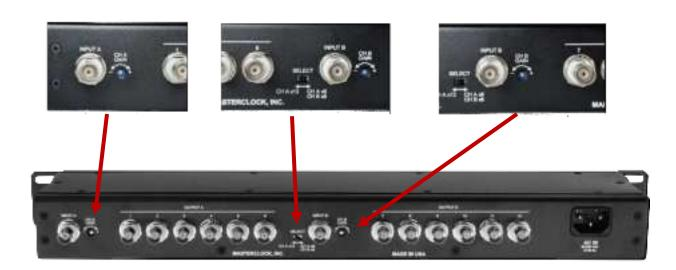
The Select switch will allow you to output channel A with a single input across all 12 outputs, or use channels A and B with their respective inputs and outputs independently.
