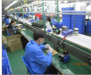
Photo of non-conformity NC 7.6 and 7.7 Worker with improper mask and No LEV.jpg
