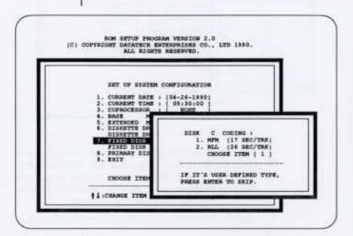
The fixed disk controllers that use the MFM and RLL encoding methods are supported. Fixed disk drives with 17 or 26 sectors per track may be configured with an MFM or RLL controller.
