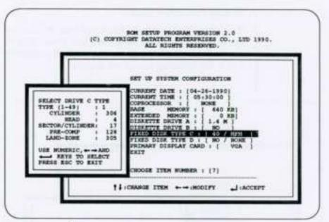
The prompt will ask what type of hard disk you have installed. There are 47 possibilities. The hard disk information screen shown above is used to indicate the type number for your hard disk. The most common types are given at the beginning of the list.
