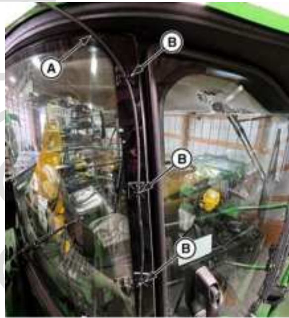
Antenna Cable Routing
