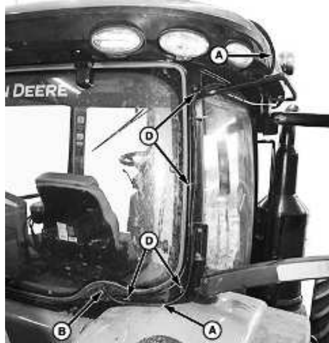
Route Antenna Cable—Corner Post
