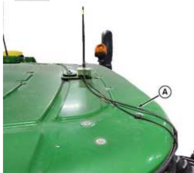
Route Antenna Cable—Cab Roof
