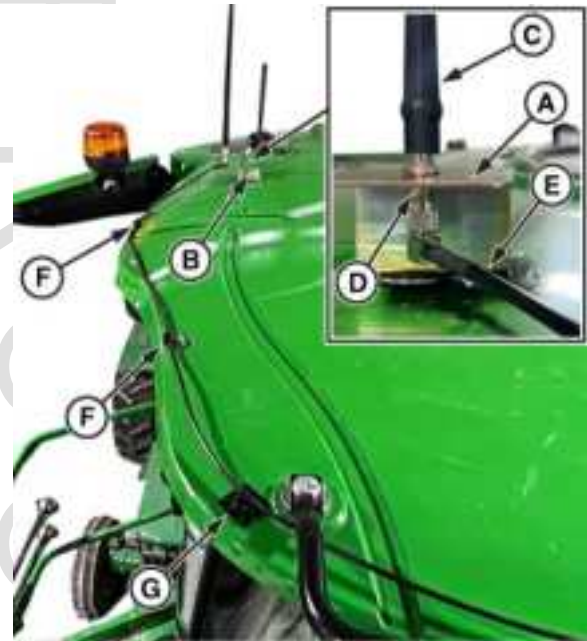
Antenna Bracket Installation
