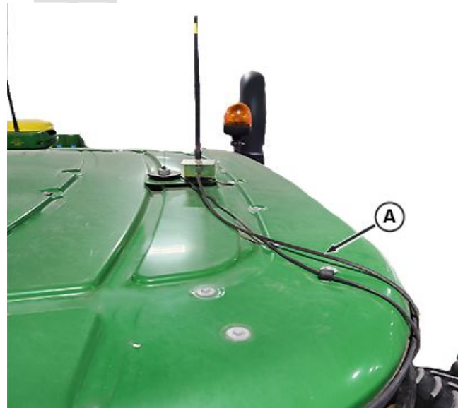
Route Antenna Cable—Cab Roof
