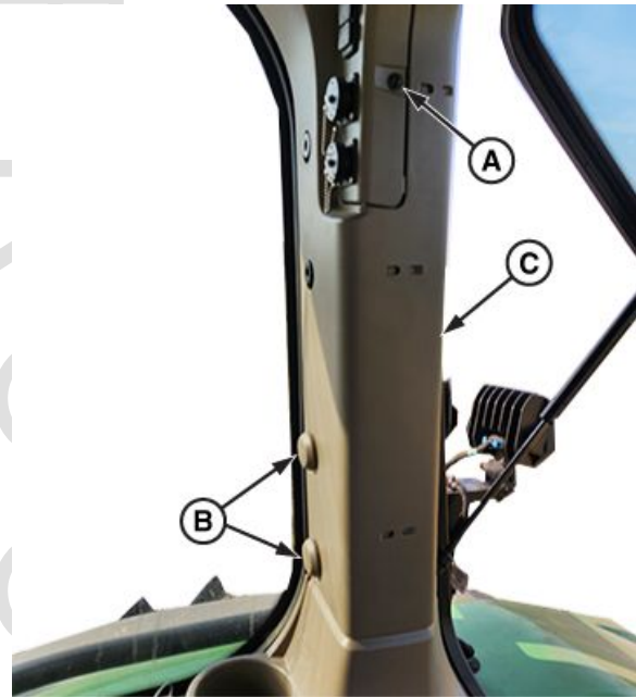
Left Rear Pillar Cover Removal
