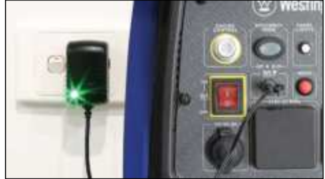
Figure 17 Connect the Battery Charger to Mains Power Supply
