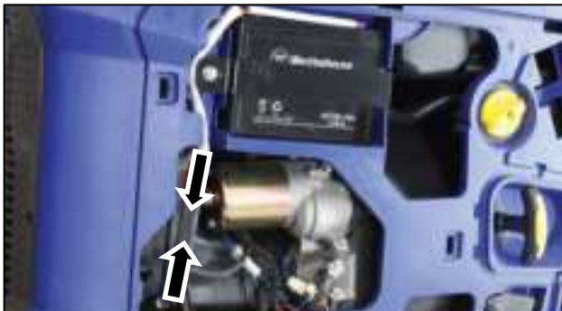
Figure 6 Assemble the Battery Wiring Harness Connector
