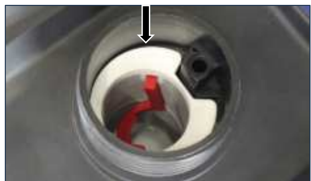
Figure 34 Install the Fuel Strainer
