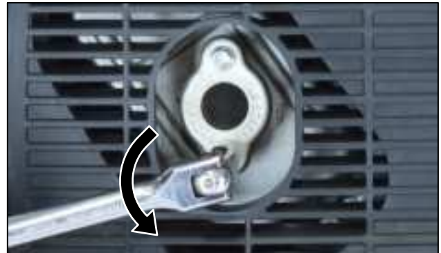
Figure 43 Remove the Spark Arrestor Clamp
