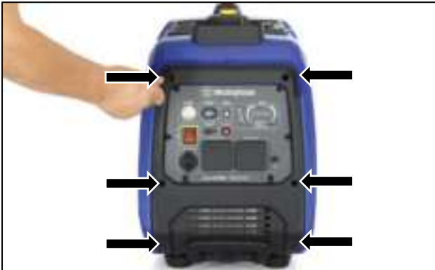
Figure 37 Remove the Front Cover Assembly
