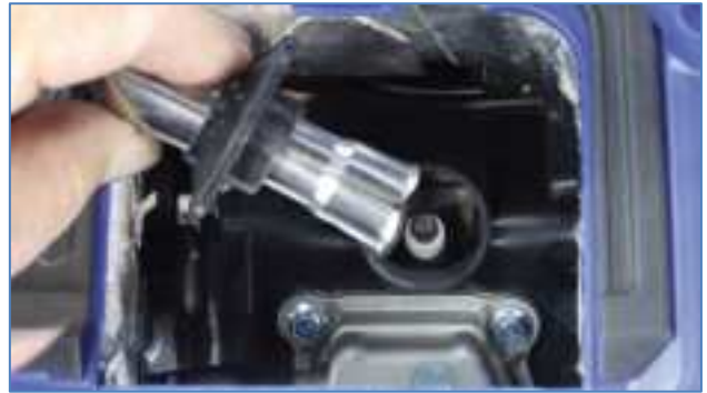
Figure 40 Remove the Spark Plug Boot
