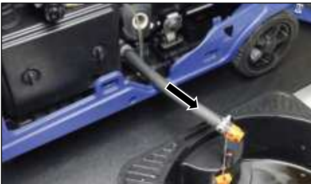
Figure 30 Draining the Engine Oil
