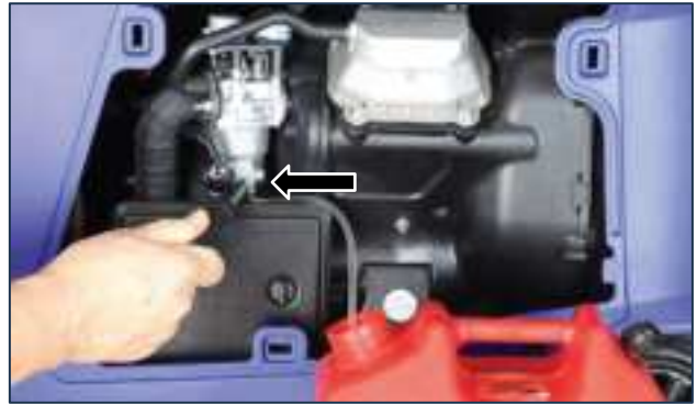
Figure 36 Drain the Carburettor
