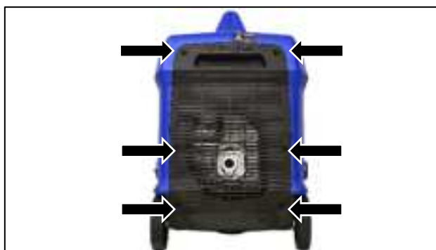
Figure 25 Remove the Muffler Access Cover
