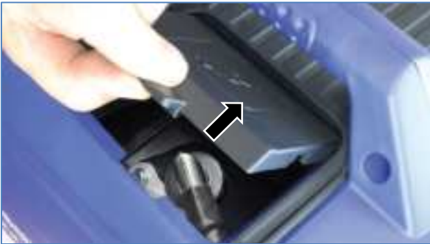
Figure 39 Remove the Spark Plug Access Cover
