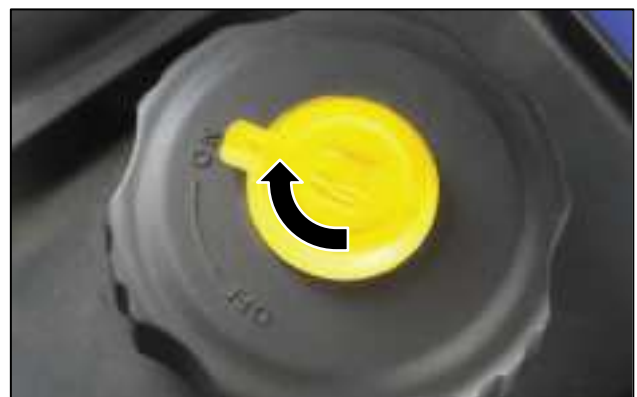
Figure 7 Fuel Cap Vent in the ON Position
