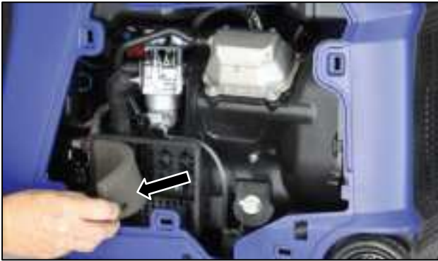
Figure 32 Remove the Air Filter Element
