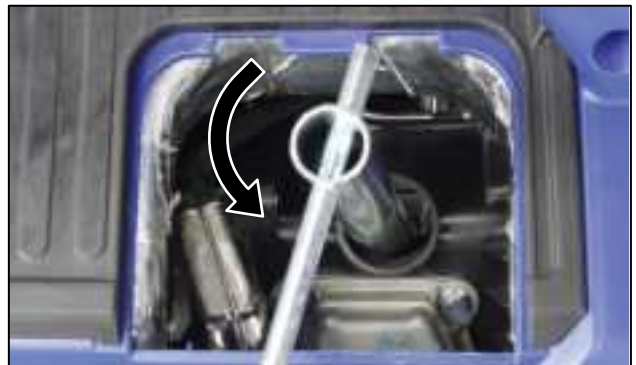
Figure 41 Remove the Spark Plug
