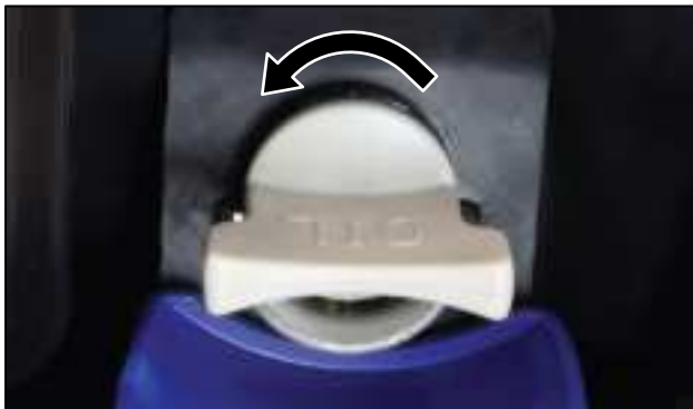
Figure 26 Remove the Oil Fill Plug
