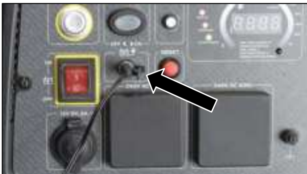
Figure 16 Connect the Battery Charger to the Generator
