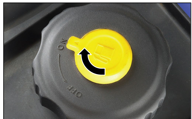
Figure 7 Fuel Cap Vent in the ON Position
