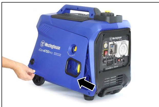
Figure 24 Remove the LHS Access Cover
