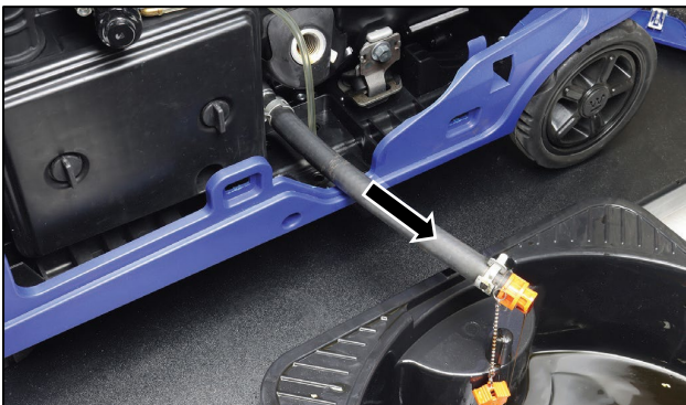
Figure 30 Draining the Engine Oil
