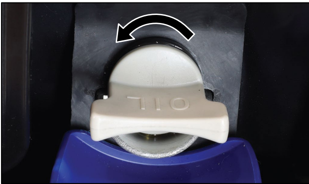
Figure 26 Remove the Oil Fill Plug
