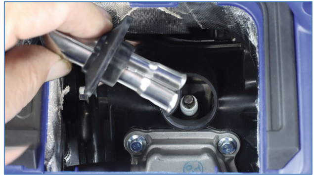
Figure 40 Remove the Spark Plug Boot
