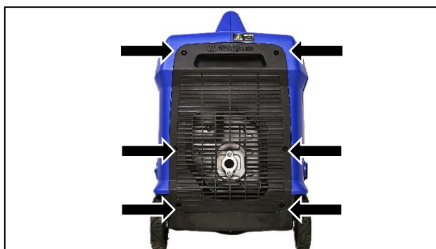
Figure 25 Remove the Muffler Access Cover
