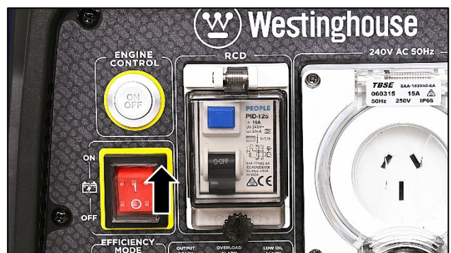
Figure 10 Battery Control Switch and Engine Control Button
