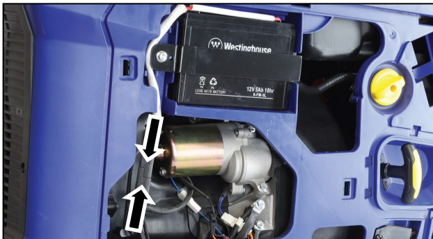
Figure 6 Assemble the Battery Wiring Harness Connector
