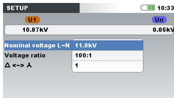
Figure 4.13: Voltage ratio for 11 kV / 110 kV transformer example
