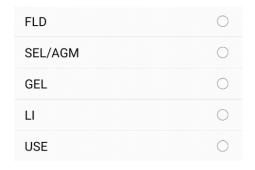
When you select battery type LI or USE, the system will allow you to set the Battery System Voltage to any of the following parameters: 12V / 24V / 36V / 48V. "AUTO" option is not available for these battery types.
