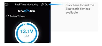
On the right-hand side, you will see a slide menu displaying the Bluetooth IDs of nearby devices, ranked by signal strength. If you don't know your device ID, just connect to the device with the strongest signal.
