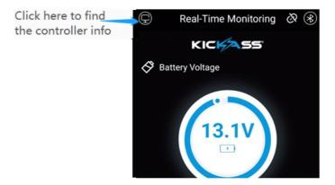
On the left-hand side, you will see a slide menu displaying device information including Bluetooth ID, Controller Model Number (original), and Device Firmware Version Number. You will also see options relating to:
