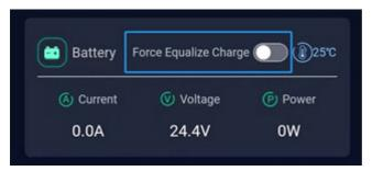
Please note that once you tap "CONFIRM" in the dialogue box, the charge cannot be cancelled. If you have made a mistake and do not want to initiate a Force Equalize Charge, disconnect both the PV and battery connections from the controller, and also disconnect the Bluetooth device from the app. When you reconnect everything, you will find the switch has reverted to the "off" position.
