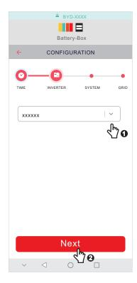
7. Choose the battery system model, HVL. And then, set how many battery modules are installed per tower.
