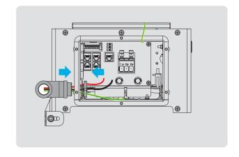
6. Loose the nut on the grounding post, put the PE terminal through it, and fix the nut again with a cylinder screwdriver (8 mm) (5/16 in), and tighten it (torque, 4 Nm/ 35.4 lbf· in).
