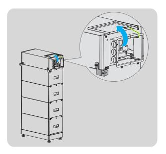
4. Remove the original plastic cover from the bottom hole.
