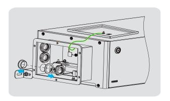
5. Get the cables through the conduit, and fix it on the BCU.
