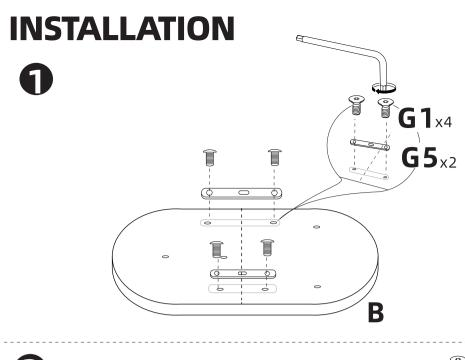
The bottom connecting iron piece G5 has a distinction between obverse and reverse sides, with the smooth side facing the ground and the flat side facing the wooden board.
