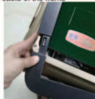
Step 9: Install the edge cover
