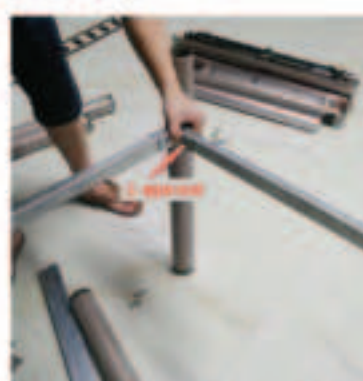
Step 3: Install the crossbars of the legs
