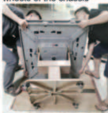
Step 5: Install the folding feet and lift the machine
