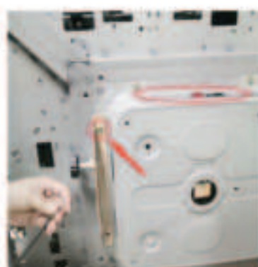
Step 3: Install the universal wheels of the chassis
