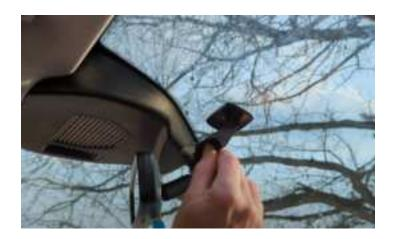
2. Use an alcohol based wipe to clear the area of the location the sensor will be installed.
