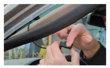
9. Use a cable tie to secure the connection and trim any excess tie.
