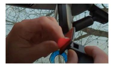
5. Slide the sensor unit into the bracket and use the provided locking tool to tighten the unit in place, ensuring the sensor is facing level and forward.
