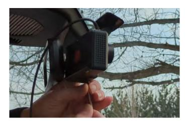
6. Route the cable between the headliner and roof towards the A pillar. Remove the door gasket and cover on the A pillar so that you can route the cables underneath the curtain airbag.
