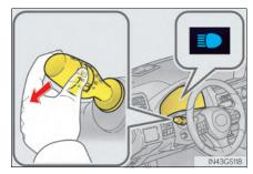
**2** Press the Adaptive High-beam System switch.
