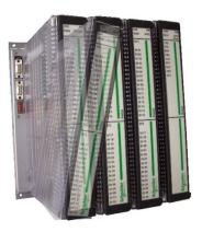
The SM\_BPX module has two fixing flanges located at the upper and lower parts respectively. There are several drill holes of 4 mm in diameter for wall or panel fixing. The number and location of the drill holes depending on the model, 6 in the SM\_BPX4 and 8 in the SM\_BPX9.
