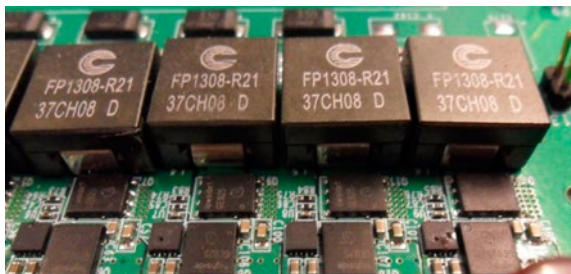
Example: High performance Server (PCB: 8 layer, 70μm)
