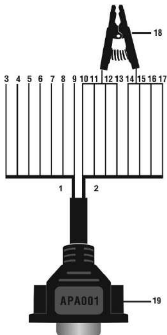
Figure 2-5 EEPROM Clamp Integrated MC9S12 Cable
