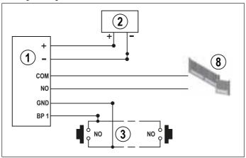
8 Gate connection to "NO" of the relay output used and to "COM"; it may also be useful to use both relay outputs, e.g. relay output #2 for the gate and relay output #1 for the door connected.
