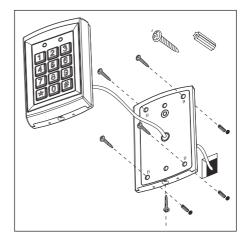
The wall mount must be fitted so that the opening for the locking screw (E) faces downwards.
