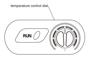
Once your freezer is in its proper place, plug the power cord into an electrical socket to turn on the unit. The light (green) will be lit if the freezer compressor is in operation (i.e., the temperature control dial is set anywhere from 1 to 7).
