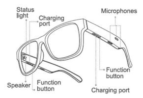
**NOTE:** The left and right function buttons perform the same tasks and can be used interchangeably.
