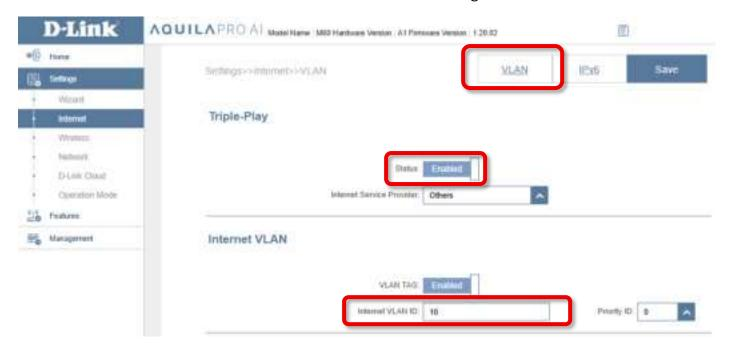
• Configuration for VDSL type of connection:
