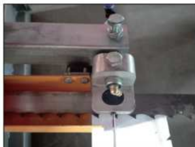
Adjust the gap below the saw blade.
