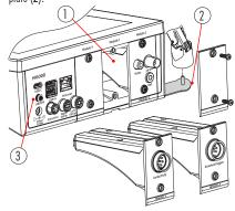
C. Connect the external stirrers (magnetic or overhead), electrodes and power adapter to rear panel of the meter.
