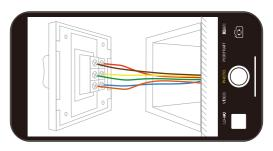
• Follow the wiring diagram to connect the switch wires to the wires in the wall box with the wire conductors.
