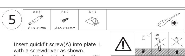
Fix part(S) to plate 1 with screw(F) as shown.
