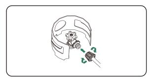
2. Fully open the Propane/LPG cylinder knob.
