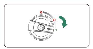
**Note:** For restarting a warm engine, turn the starting dial switch directly to the "RUN" oposition.
