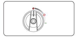
3. Turn the cylinder valve to the "OFF" position.
