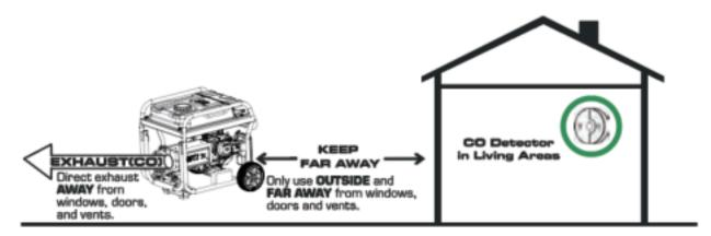
However, if the generator misused and operated in a location that results in the accumulation of CO inside an enclosed or partially enclosed space, CO WATCH- GUARD automatically shuts off the engine and notifies the user of what has happened and directs the user to read the instruction of CO WATCH-GUARD Action Label for steps to take.
