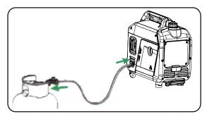
4. Open valve on propane LPG cylinder and check all connections for leaks by wetting the fittings with a solution of soap and water. Bubbles which appear or bubbles which grow indicate that a leak exists. If a leak exists at a fitting, then turn off the valve on the cylinder and tighten the fitting. Turn the valve back on and recheck the fitting with the soap and water solution. If the leak continues or if the leak is not at a fitting, then do not use the generator and contact customer service.
