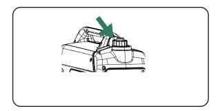
3. Turn the fuel cap vent lever to the "ON" position.
