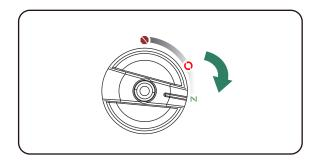
**Note:** For restarting a warm engine, turn the starting dial switch directly to the "RUN" oposition.
