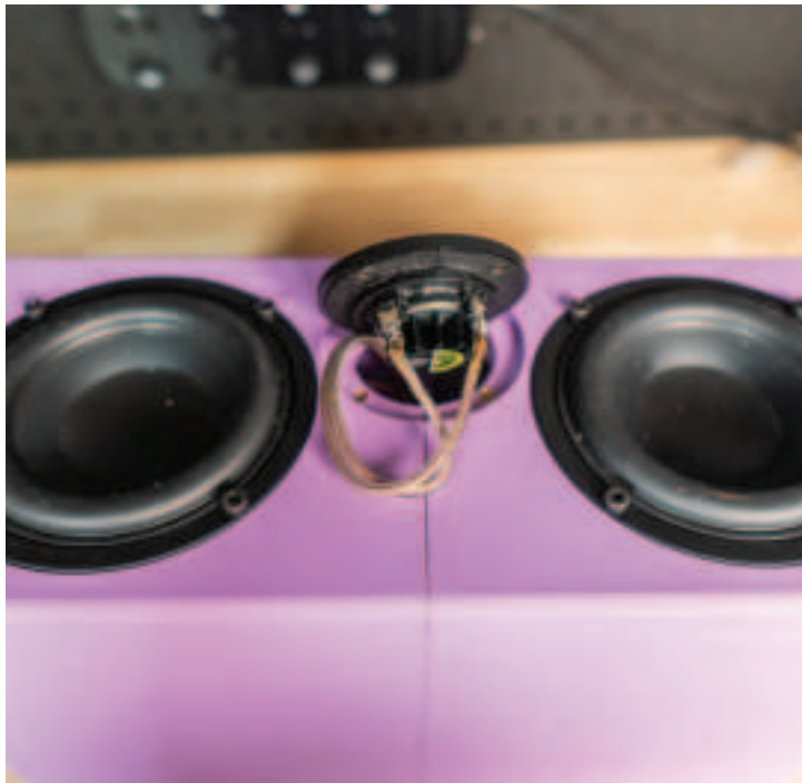
• Make the Connection: Solder the wires to the contacts on the tweeter. Pay close attention to polarity.
