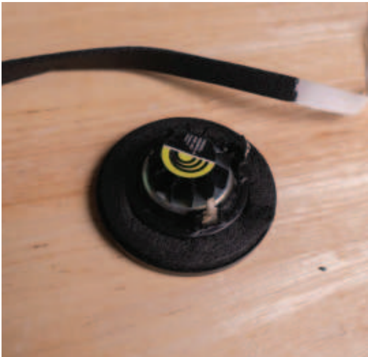
• Tape It Up: Looks like Dayton skimped on the gasketing tape! Layer up the back of the mounting surface of the tweeter with some extra. Without a tight seal, the sound suffers big time.
