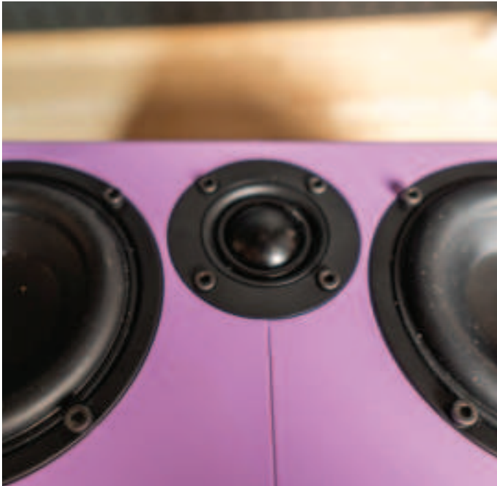
• Driver's Seat: Screw the tweeter in place, nice and secure. Ensure not to over tighten the screws.
