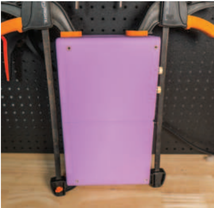
• The Clamps: Clamp the two enclosure halves together and set aside while the glue sets.
