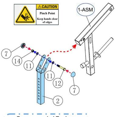
TIP: Fully tighten HEX BOLT (12) then loosen the locking NYLON NUT, THICK (14) approximately 1/4 turn so that the LEG WEIGHT HOLDER - Assembly (1-ASM) & ADJUST TUBE (2) pivot freely with little to no excessive movement
