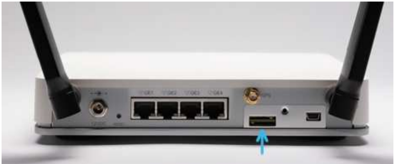
Figure 2. Insert SIM card
