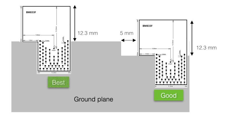
We don't recommend mounting BM833F/BM833AF module in the middle of a host PCB.
