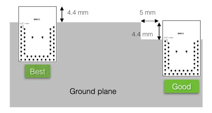
We don't recommend mounting BM833 module in the middle of a host PCB.
