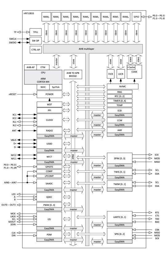
following is a diagram of Nordic nRF52833 SoC.
