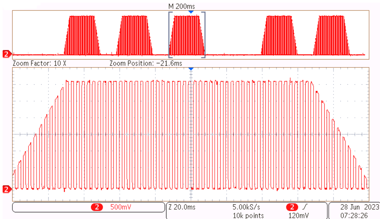
Figure 3-1. High-Alarm State DAC Waveform
