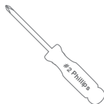
Tools to remove cover of indoor unit
