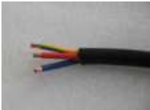
▲ Figure 4.15 Stripped AC Wires
