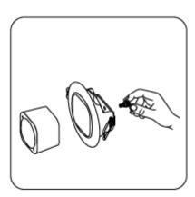
3. Bend in Recessor holder and fit Recessor into the ~75mm / 3" hole then release.
