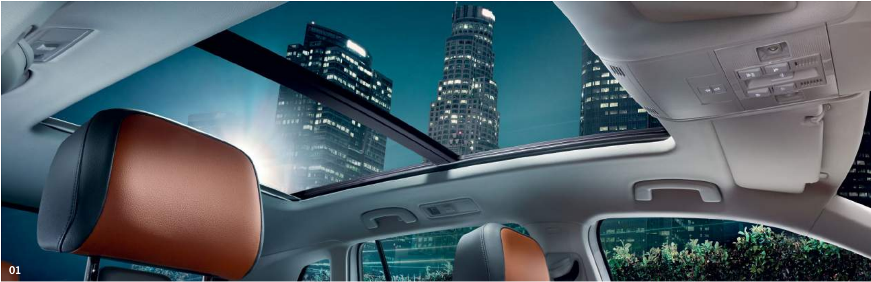
01 The electrically operated, panoramic glass sunroof with integrated roller blind adds additional light and space, whether open or closed, filling the interior with natural light and providing an inviting view of the sky above, and when tilted upwards it lets in fresh air. Image shown is Tiguan SEL with optional 'Vienna' leather upholstery.
