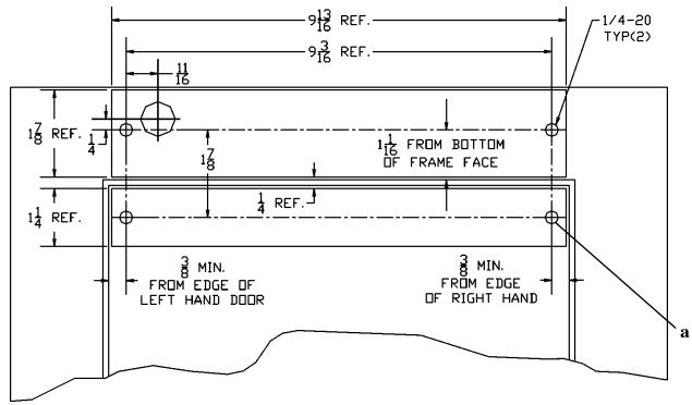
NOTE: Hole (a) - size and type depends on door type and mounting style.
