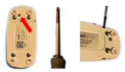
2. . Insert an AA Battery in the sensor and close the cover. Note: Insert first the black jack in the hole (cover) of the sensor.
